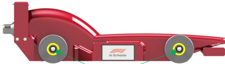
View of wheels only obstructed by wheel support system (circled in yellow)
