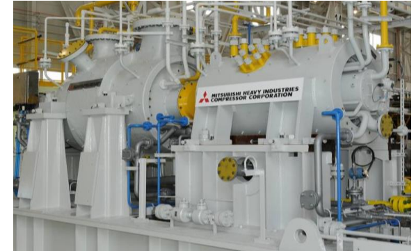
Compressors for FPSO
