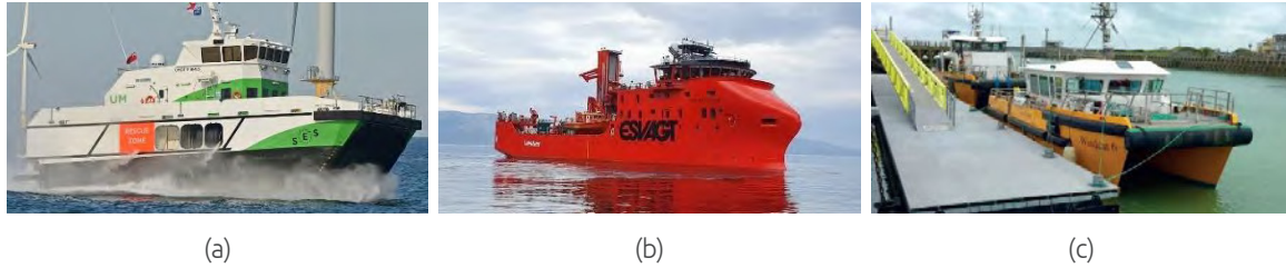
FIGURE 18 – Service vessels: (a) Crew transfer vessel, (b) Service operation vessel, and (c) Guard vessel (Ramboll, 2022).
