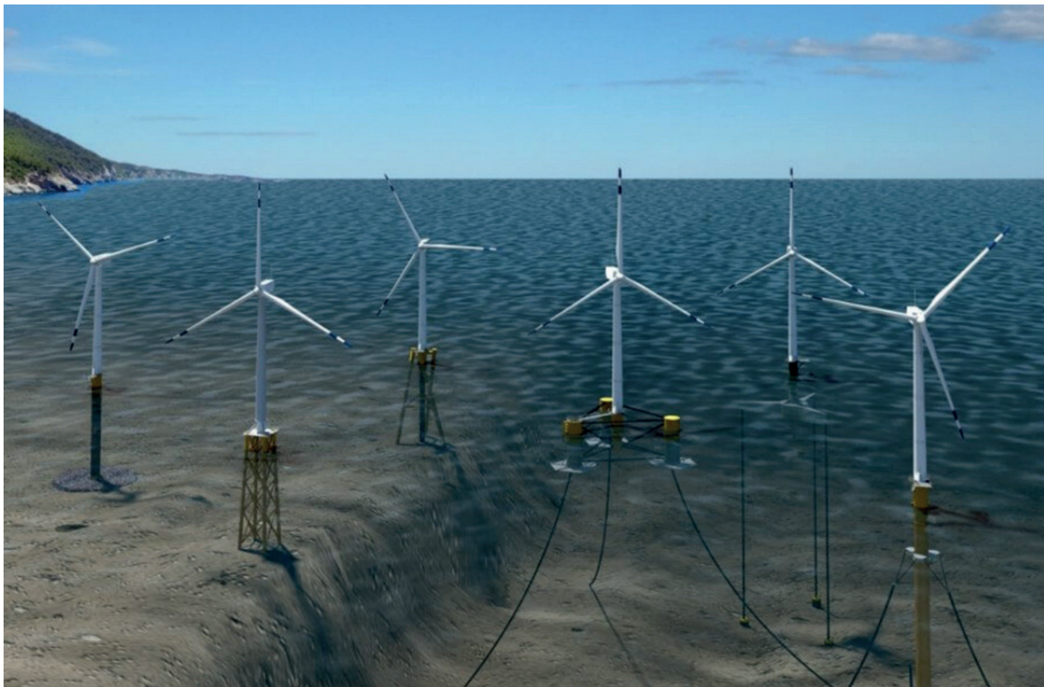
FIGURE 15 – Types of offshore wind power foundations.
